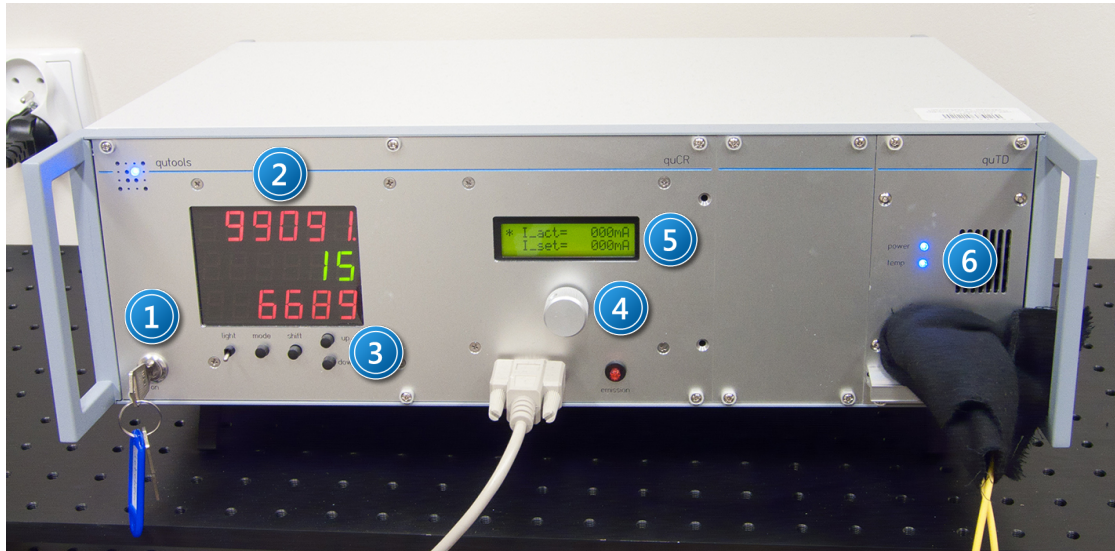
Picture 7. Measuring unit – controller, multifunction power supply, single-photon detector: 1 – main switch; 2 – count display; 3 – count function keys; 4 – laser settings dial; 5 – laser settings display; 6 – APD module indicators.
